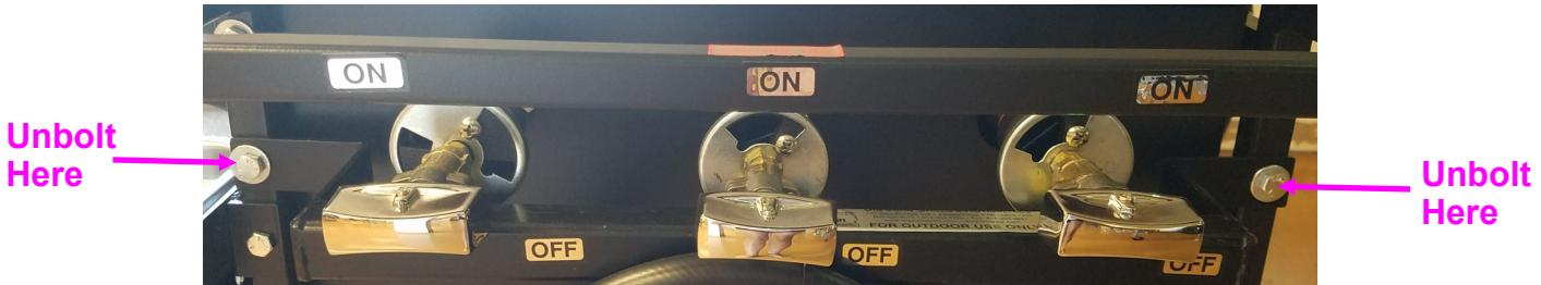
2. Gently lift manifold away from griddle body - careful not to rip it off as the orifices of the control valves are inserted into the silver disk portion of the air mixer.
